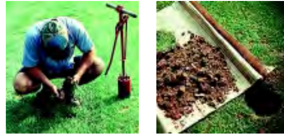
Sampling with the cup-cutter (bulb-planter) method.
